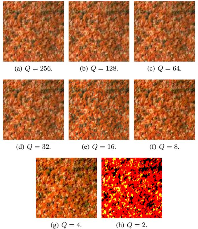
Fig. 3. Uniform color quantization of the image 3(a) coded in the  $(R, G, B)$  color space.
