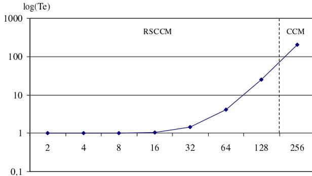
Fig. 6. Mean computation time  $T_e$  (in millisecond) required to extract a feature, from an OuTex image whose size is  $128 \times 128$  pixels, according to the quantization level  $Q$ .
