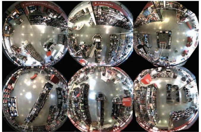
Fig. 7. The scene, as it is seen by the six fisheye cameras of our system. Due to the high number of occluders and the low resolution ( $240 \times 240$  pixels) of each camera view, distant zones are not easily perceived.
