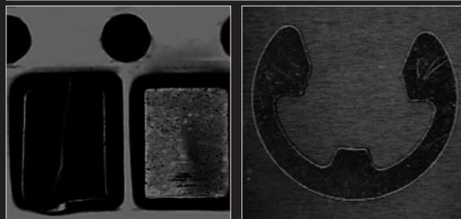
An irregular surface is photographed dark, because it does not reflect light to a camera when irradiating a work with coaxial light with a camera.
