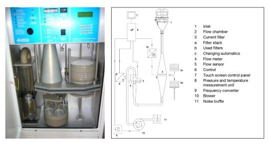
Figure 8. Digitel DA80 high volume sampler used for data acquisition (source of the right plot: Digitel).
