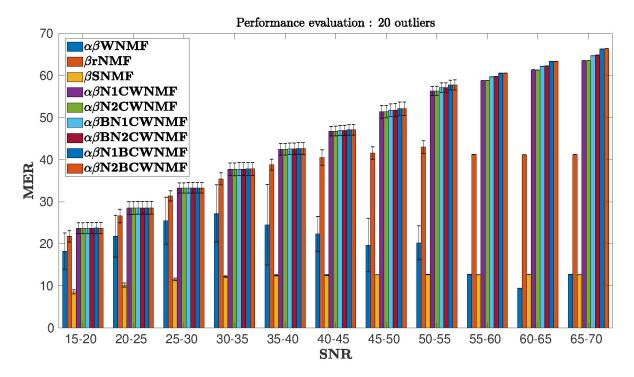
**Figure 5.** MER vs. input signal-to-noise ratio (SNR). The case with 20 outliers.
